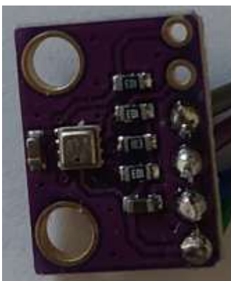
A BME280 type temperature, humidity and atmospheric pressure measurement module.
