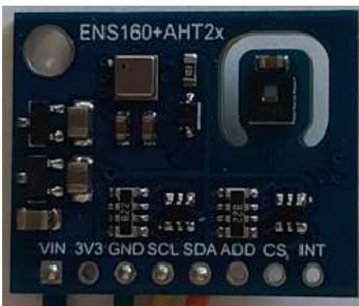
An ENS160 pollution and air quality measurement module, QA, Tvoc, Co2 measurement associated with an Aht25 sensor measuring temperature and hygrometry for the calibration of the ENS160 module.
