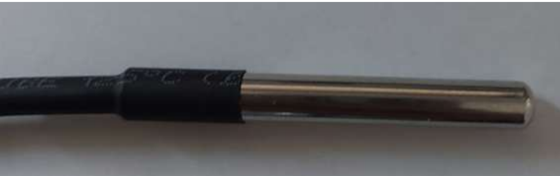
DS18B20 type remote temperature sensors encapsulated in stainless steel.
